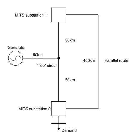
The intact marginal cost for this generator is first established. This calculation is performed by the transport model, although it is repeated by the seculf program. An additional MW of generation is added at the generator node and an additional MW of demand is added at the slack node (in this case MITS substation 2). This causes the additional powerflows shown as "intact" in the diagram below.
