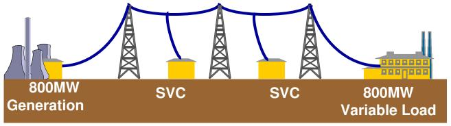
SVCs dynamically regulate the network by providing or absorbing reactive power.
