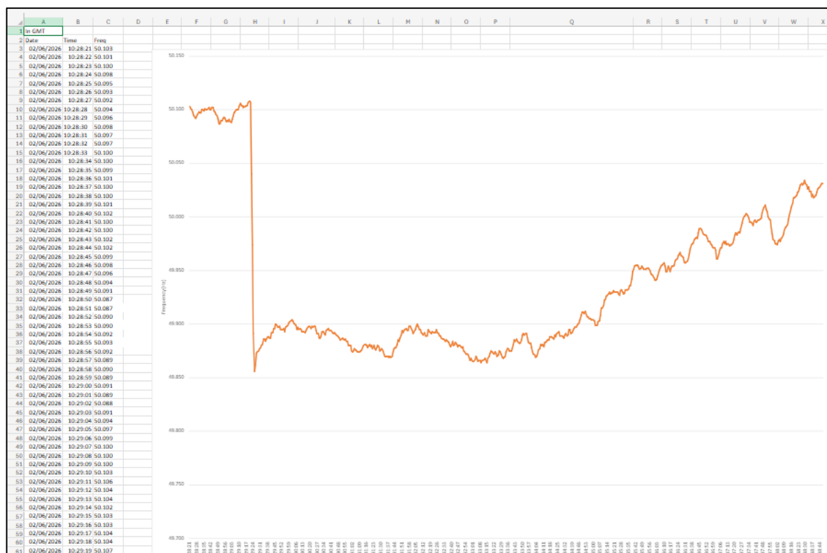
Figure 04: GC0151 and GC0105 System Incidents Report June 2026, '20260602-1' Tab, displaying System frequency trace (1-second interval) for a specific incident which occurred on 2 June 2026.
