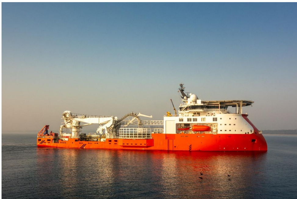
Figure 5.9: A typical cable-laying vessel
