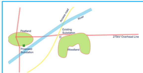
Figure 16: Substation located on the edge of peatland
