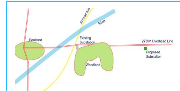
Figure 18: Substation located outside of a flood risk zone
