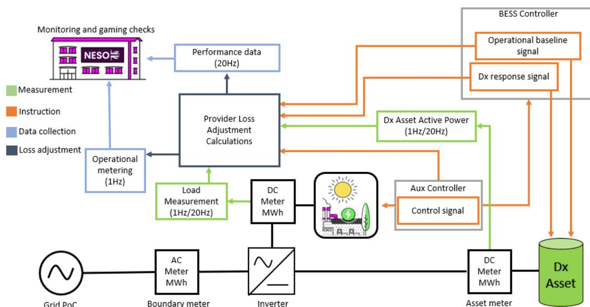
Figure 6: Diagram of information and energy flows for Solution 3 sites.
