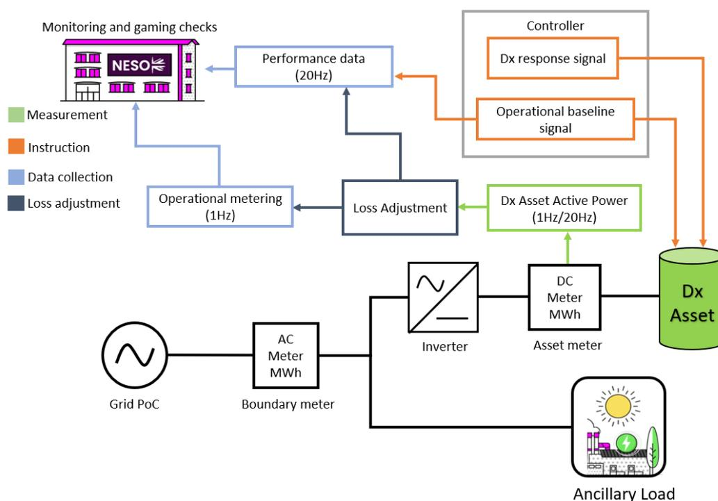
Figure 5: Diagram of information and energy flows for Solution 2 sites.
