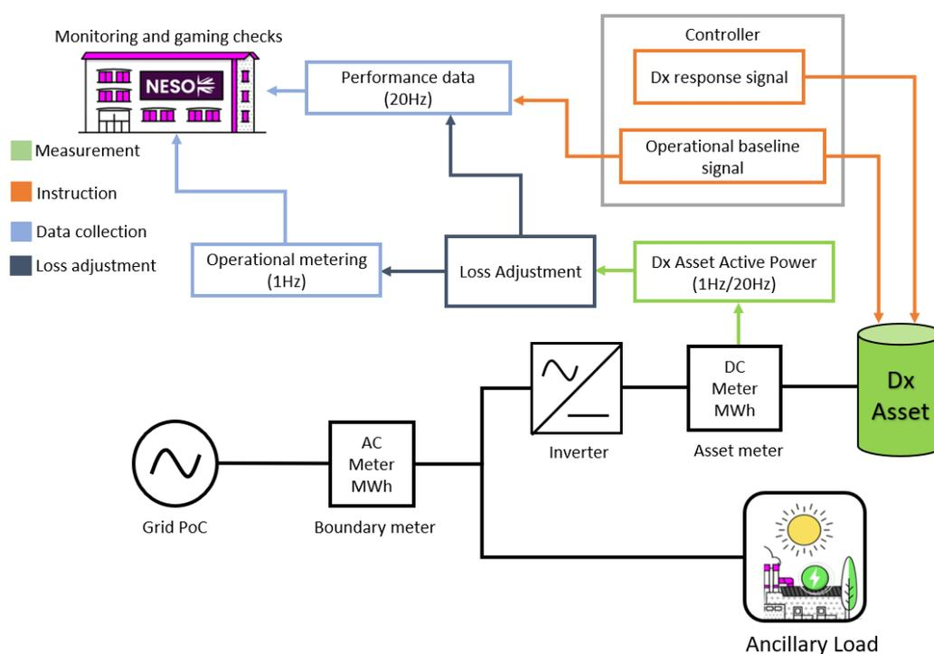
Figure 3: Diagram of information and energy flows for Solution 2 sites.
