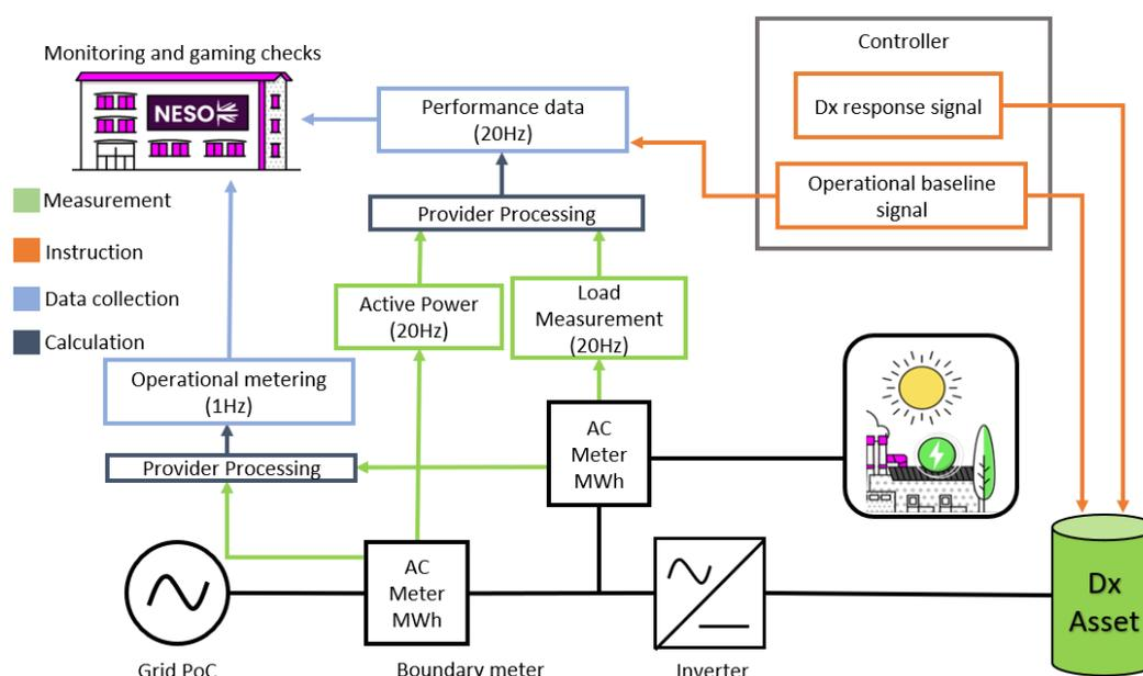
Figure 2: Diagram of information and energy flows for Solution 1 sites.
