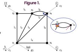
Power flow is then modelled across this topology, solving for continuous variables such as active power (for DC and AC) reactive power and voltage, (for AC), and dispatch (for optimal power flow [OPF]), all in the context of the chosen objective.
