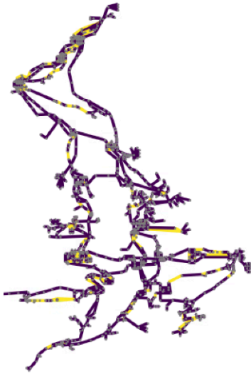
Figure 16 - Candidate pipes for removal are highlighted within the graph network - where our initial iteration identifies “redundant segments” between bifurcation in the network.
