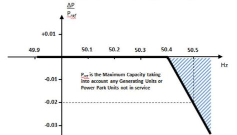
Active Power Frequency response capability of when operating in LFSM-O
