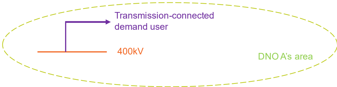
Figure 2 Assigning demand zone for a transmission-connected user
